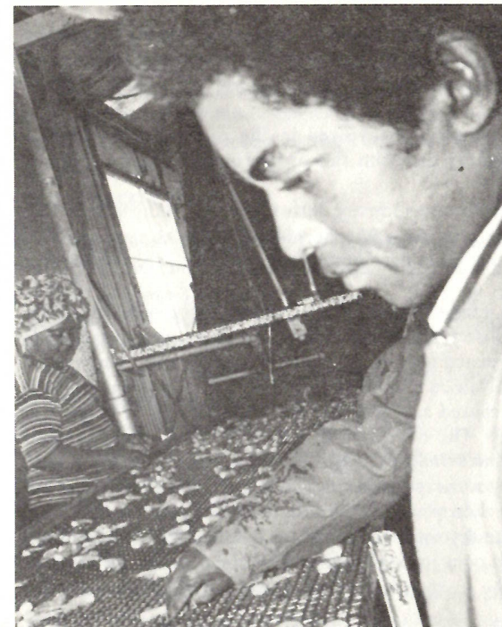
Culling the shrimp as they move along the conveyor belt to remove any remaining foreign materials.
