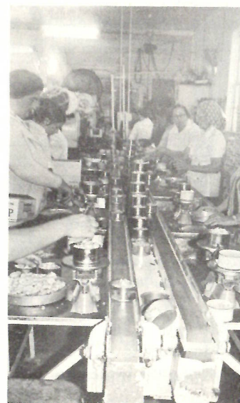
Company assembly line where shrimp are weighed & packed in cans.
